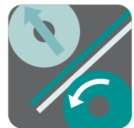
Compound paper being fed by releasing the Double-Feed Prevention Roller.
