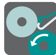
Compound paper being fed without releasing the Double-Feed Prevention Roller.
